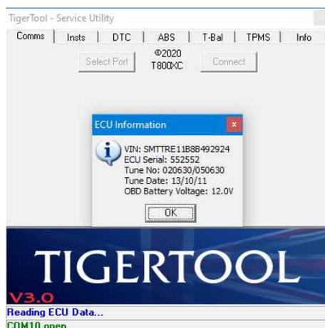
If the ECU type-check matches and data was read successfully, the 'ECU Information' pop-up box should appear, as shown above, to display the VIN number, ECU serial number, engine map/tune number, the date the tune was installed, and the approximate battery voltage.
