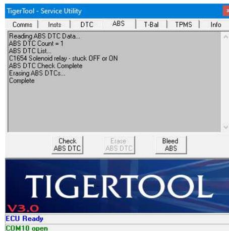
After erasing ABS DTCs it may also be necessary to re-check & erase non-ABS DTCs as some are inter-linked. You may also need to switch off the ignition, wait 1 minute then switch on again to allow the ECU and other systems to fully reset before re-checking for ABS DTCs.
