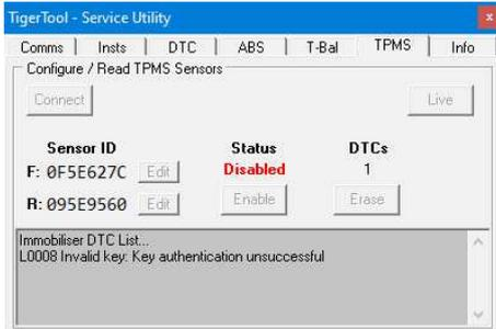
This error is caused by the immobiliser not responding to the TPMS Enable command.
