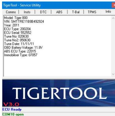
If the immobiliser is not found, as would be the case if the bike is equipped with a Chassis ECU, the following image should appear:-
