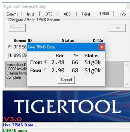
The status labels will indicate if there is a problem with either tyre sensor data. In the images above the normal signal status is shown.
