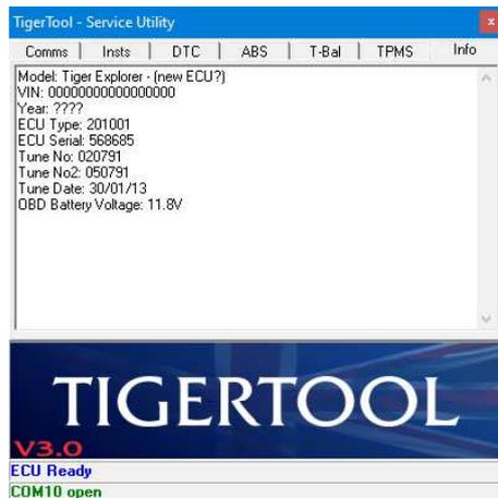
The model info is selected from a list based on the VIN. In the case of Explorers that have had their ECU replaced under recall (Triumph SB505), the VIN may read all zeros making it impossible to decode, so the Model will appear as shown in the second image.
