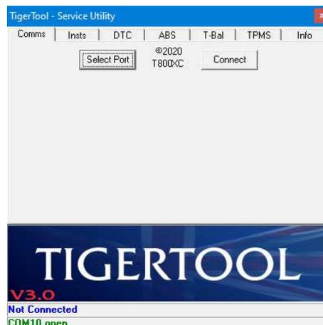
Now click the 'Connect' button to start communicating with the ELM327 interface and ECU - this may take several seconds and should indicate progress according to the following images:-
