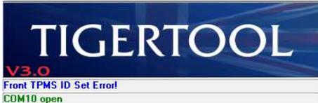
This error is caused by a timeout while waiting for confirmation that the new sensor ID has been stored in the immobiliser. The sensor ID was accepted but not confirmed.
