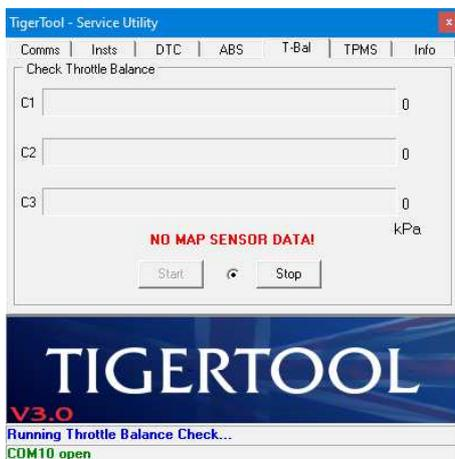
This can be caused if the engine is not running, or your MAP sensor is disconnected.
