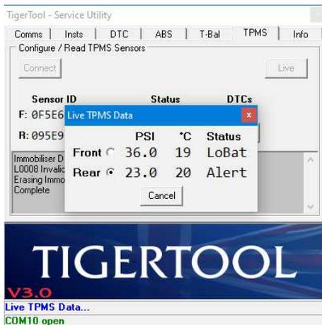
In this image the rear tyre sensor is reporting a low tyre pressure alert. The TPMS warning light should also be displayed on the bike's instruments.
