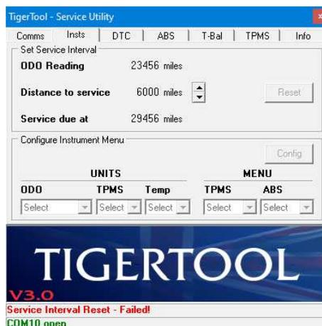
As with other diagnostic features, the most likely cause of this error is the bike's ignition or engine kill switch being in the off position. Ensure that the both switches are on and try again.
