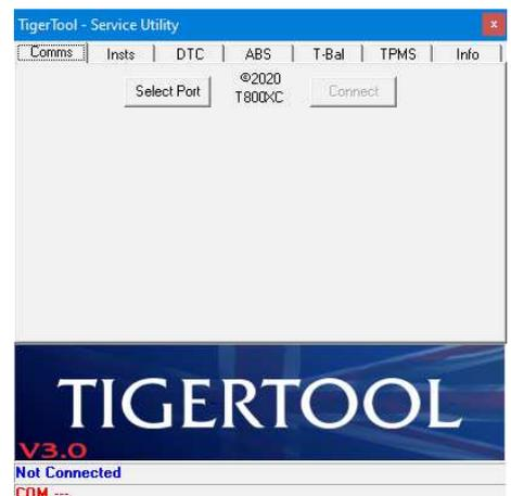
Click on the 'Select Port' button then use the arrow in the list box to select the serial port for your ELM327 interface. Depending on your PC configuration you may have several serial ports so it's worth looking at Windows Device Manager to check which one is assigned to your ELM327 interface. In the case of Bluetooth interfaces, there may be two assigned serial ports (depending on the drivers) so you may have to try both to see which one provides access.
