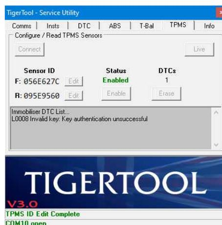
Once the new ID has been programmed into the immobiliser it is read back out again for confirmation. If successful the 'TPMS ID Edit Complete' message should be seen as shown in the 4<sup>th</sup> image above.
