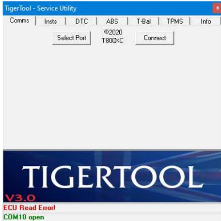
The most likely cause of this error is the bike's ignition or engine kill switch being in the off position. Ensure that the both switches are on and try again.
