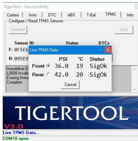
The pressure, temperature and status data for the front & rear pressure sensors will be displayed. The flashing dots near the 'Front' & 'Rear' labels are there to indicate that live readings are being taken.
