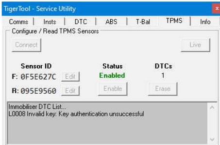
After the new sensor ID has been saved it is read back from the immobiliser to check that it matches the number that was edited. This error is caused by a mismatch between the two numbers.
