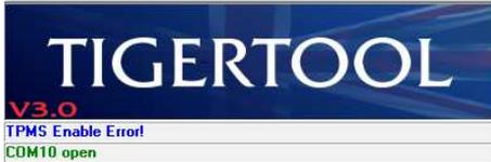
This error is caused by a timeout while waiting for confirmation that the TPMS Enabled status has been set in the immobiliser. The command was accepted but not confirmed.
