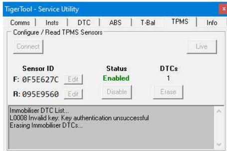
This error is caused by a timeout while waiting for confirmation that the DTC erase command has been executed.
