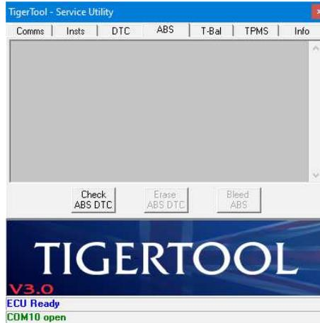
To read the list of confirmed ABS DTCs, click on the 'Check ABS DTC' button and the following images should appear if no DTCs are found. The image on the right shows the 'Bleed ABS' button has been enabled because no ABS DTCs were found.
