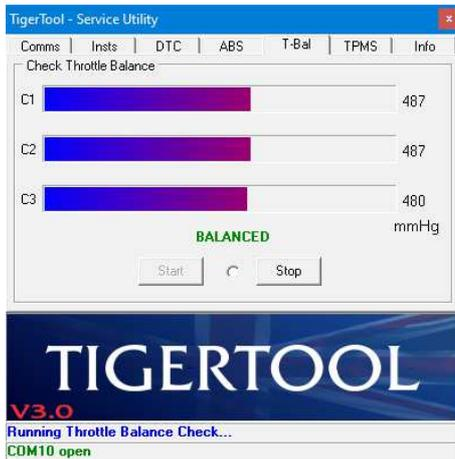
The flashing dot between the 'Start' & 'Stop' buttons is there to indicate that live readings are being taken.
