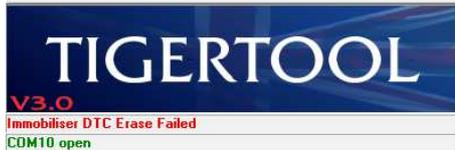
This error is caused by the DTC erase command completing but the immobiliser DTC read-back failing.
