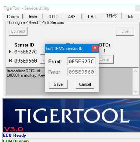
The current sensor ID for the selected tyre can now be edited. The 'Save' button will only be enabled when the full 8 digit ID has been entered. The IDs are in hexadecimal format so only characters 0-9 & A-F can be entered. The ID for the other tyre will be displayed but greyed-out to prevent editing.
