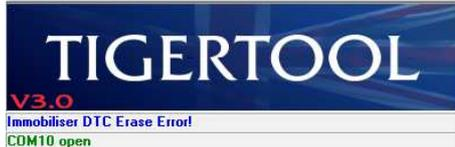
This error usually follows the one above and indicates that the DTC erase process failed.
