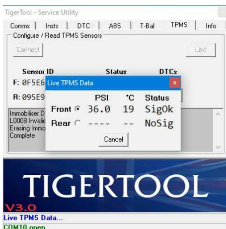
In this final image the rear tyre sensor is not transmitting any data. This message may be seen if the TPMS sensor has gone to sleep.
