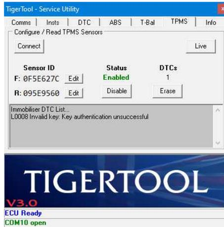
If any DTCs are found the 'Erase' button will be enabled. Similarly, if the TPMS is enabled the text on the status button will change to 'Disable' and the 'Live' button will be enabled to allow live monitoring of TPMS data (see later). Finally, if any sensor IDs are found they will be listed for the Front & Rear tyres.
