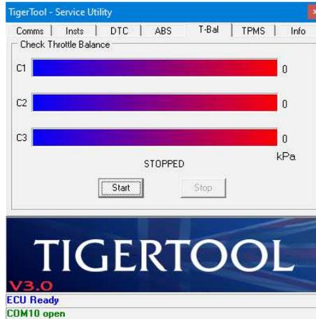
Before attempting to check the throttle balancing, start & run the engine and allow the bike to idle.
