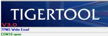
This error is caused by the TPMS Enable command completing but the status read-back suggesting that TPMS is not enabled.
