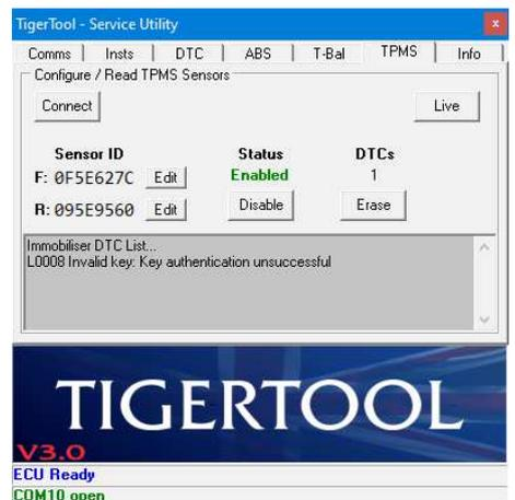
In the 4<sup>th</sup> image above, now that the TPMS is enabled, the text on the Status button has been changed to 'Disable' and the 'Live' monitor button has been enabled.
