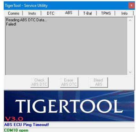
At this point the software has been disconnected from the ECU and all other TigerTool functions may have been disabled, so you'll need to re-connect to the ECU from the first 'Comms' tab to re-establish communication and to try again.
