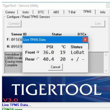
In this image the front tyre sensor is reporting a low battery voltage and the rear tyre sensor is indicating there's a change in pressure (up or down).
