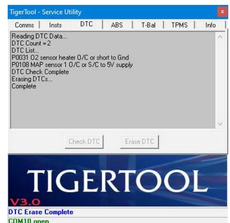
Once the DTCs have been successfully erased, you can confirm this by re-clicking the 'Check DTC' button. It may be necessary to switch off the ignition, wait 1 minute then switch on again to allow the ECU and other systems to fully reset before re-checking for DTCs.
