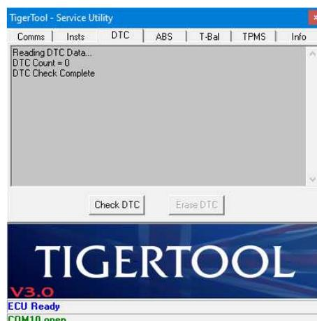
If any confirmed DTCs are found the 'Erase DTC' button will be enabled and the codes will be listed. You can scroll down through the list if there are too many to show in one pane. The following example image shows a typical DTC result list:-
