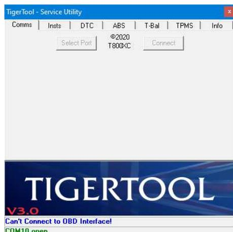
The most likely causes of this error are either the wrong serial port being selected or no power to the ELM327 interface. Try to unplug then reconnect the interface from the bike (and observe the active LEDs) and/or try a different serial port. Also make sure that the ignition & engine kill switches are on.
