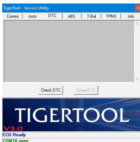
To read the list of confirmed DTCs from the ECU, click on the 'Check DTC' button and the following images should appear if no DTCs are found:-
