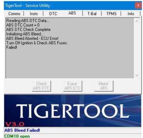
This error can be caused by a faulty supply to the ABS modulator. It usually indicates that the ABS ECU is responding but there's no power to drive the solenoids & pump sections. The ABS fuses and wiring should be checked.
