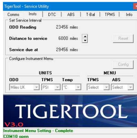
Once completed, the odometer details are re-read from the bike in case the distance units have been changed between miles & km.
