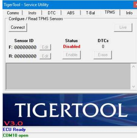
If you click on the 'Connect' button TigerTool will try to establish a connection with the immobiliser, read any stored DTCs, read the enabled/disabled status and finally read any stored sensor IDs, as shown in the following sequence of images:-
