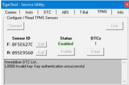
This error is caused by the immobiliser not responding to the sensor ID programming command.
